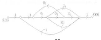
2. a) Determine the overall T.F  $\frac{C}{R}(s)$  for the system shown in Fig.
